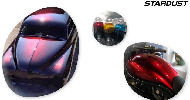
The candy color is the visual result of a **multi-layer system**, which reflects and colors the light and thus creates a **transparent**, **iridescent and luminous color**. This technique is realized with a Candy undercoat and a Candy tinted varnish. By **combining the different Candy layers**, with the different Candy varnishes, a large number of color combinations can be obtained.
